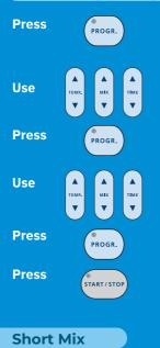
for longer than 2 seconds. Control light will light when the function is activated. On the display, the box to the left of the temperature indicates the first step of the program.
